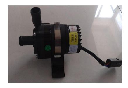
Features: small size, light weight, compact structure, wide range of applicable environments, platform development and design. Under the same shape, different speed, power and lift requirements of different vehicles can be met by PWM speed regulation. The pump has functions such as constant power, overvoltage protection, stall protection, dry running protection, reverse connection protection, and soft start.
