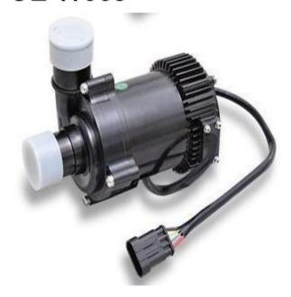
Features: small size, light weight, compact structure, wide range of applicable environments, platform development and design. Under the same shape, different speed, power and lift requirements of different vehicles can be met by PWM speed regulation. The pump has functions such as constant power, overvoltage protection, stall protection, dry running protection, reverse connection protection, and soft start.
