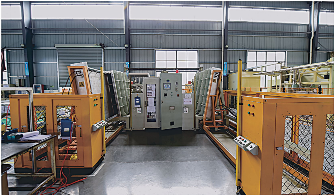
HELIUM LEAK INSPECTION MACHINE 氮检仪
