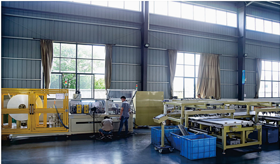
FAST FIN FORMING MACHINE AND COIL AUTOMATIC ASSEMBLE TABLE 翅片快速成型机和自动组装机
