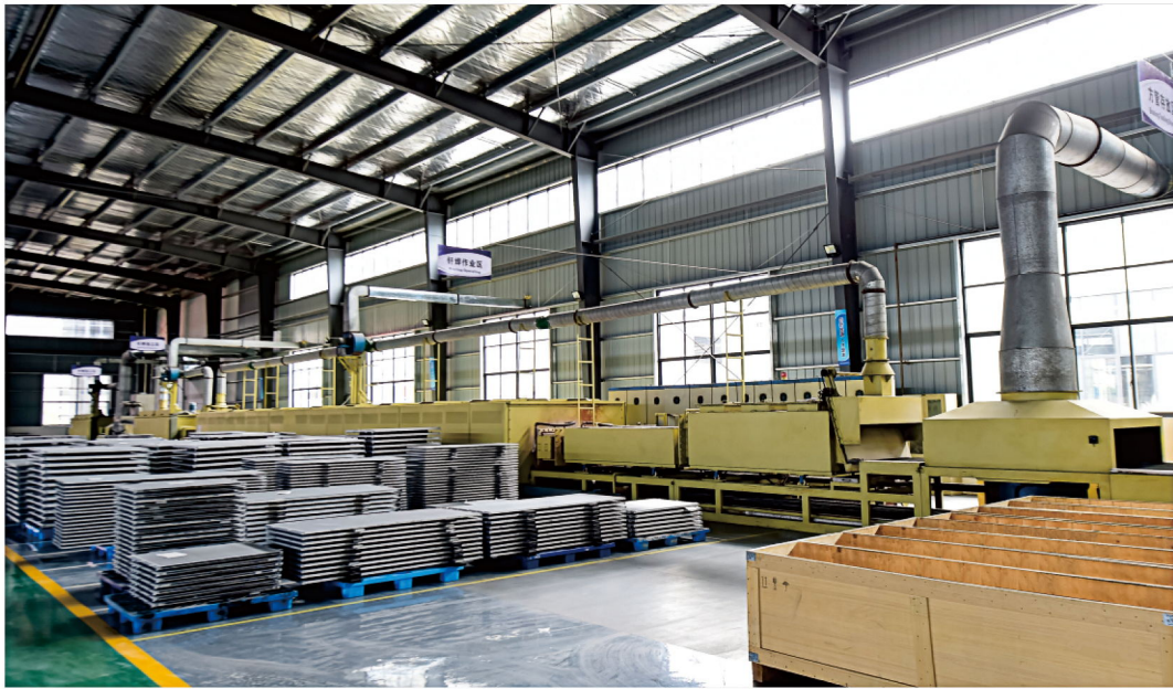
NOCOLOK BRAZING FURNACE NOCOLOK 钎焊炉
