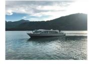
Energy: 480kWh Length: 21m 2\*45kW Power: 19km/h Speed:
