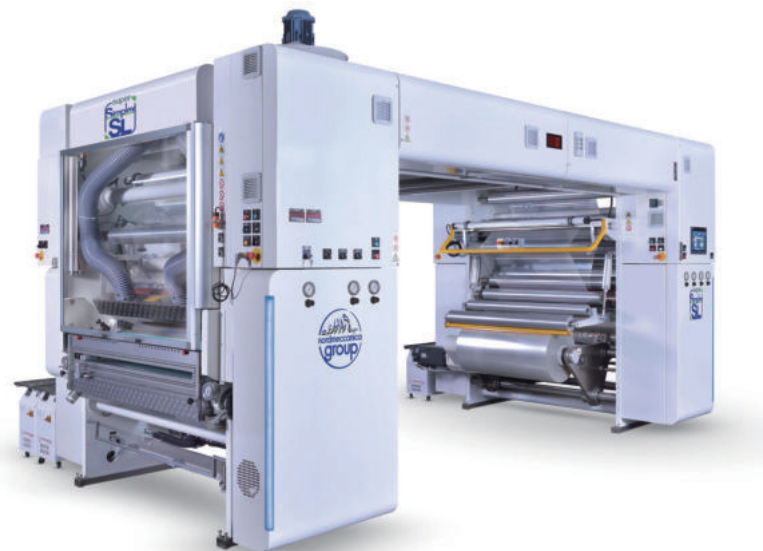
无溶剂复合Solvent-free Lamination NORDMECCANICA
