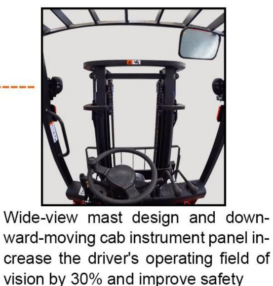
ward-moving cab instrument panel increase the driver's operating field of vision by 30% and improve safety
