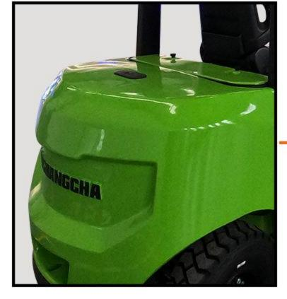
Independently developed and produced integral casting counterweight,,which is more than at least 100KG heavier than other competitors, maintaining value and more stable
