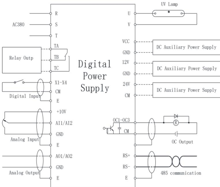
Table 2-5 Power Supply Basic Wiring Diagram
