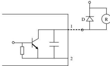
Figure 5-1 OC terminal internal circuit
