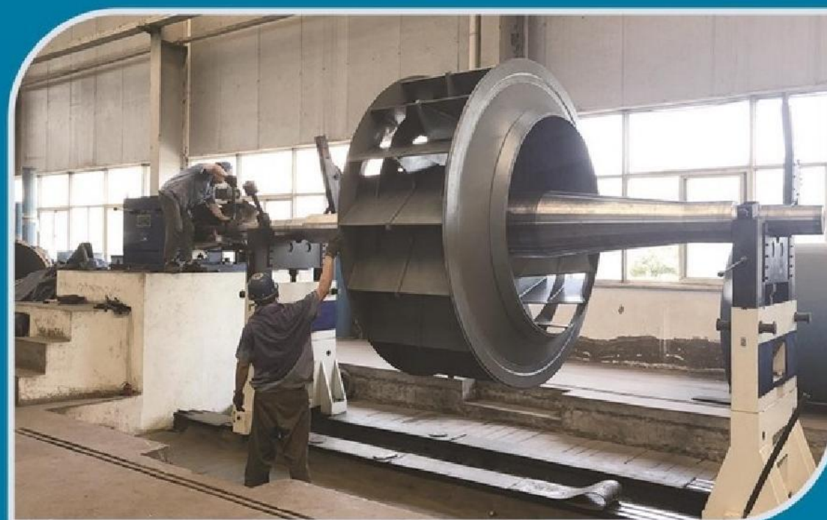
◆ 40T Dynamic balancing machine
