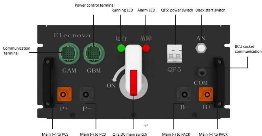
High-voltage Box Panel Layout
