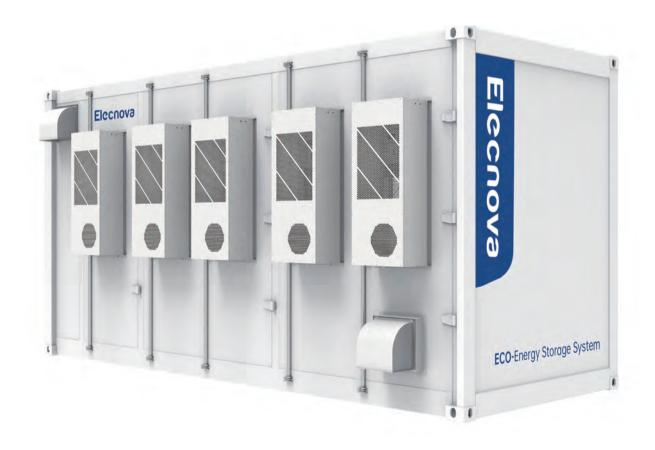
The 20-ft air-cooled ESS container product integrates PACK, EMS, BMS, HVAC, fire safety system into one container. It has the advantages of high energy density, easy transportation & installation, and high protection level. The DC output can combine with PCS-boost container to realize AC network connection at medium/high voltage. It can be applied to the generation side, grid side, and ESS applications with high power/capacity requirements.
