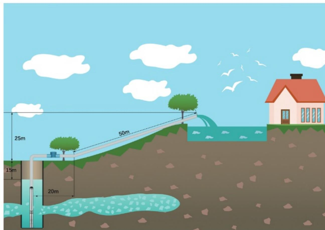
In the figure above, the H0 dynamic water level is 15m (the distance between the water surface and the ground), the flat bottom distance is 20m, the slope length is 50m, the vertical height of the H1 pool is 25m, and the H2 pipeline loss (every 100m pipeline will lose 3m of head)
