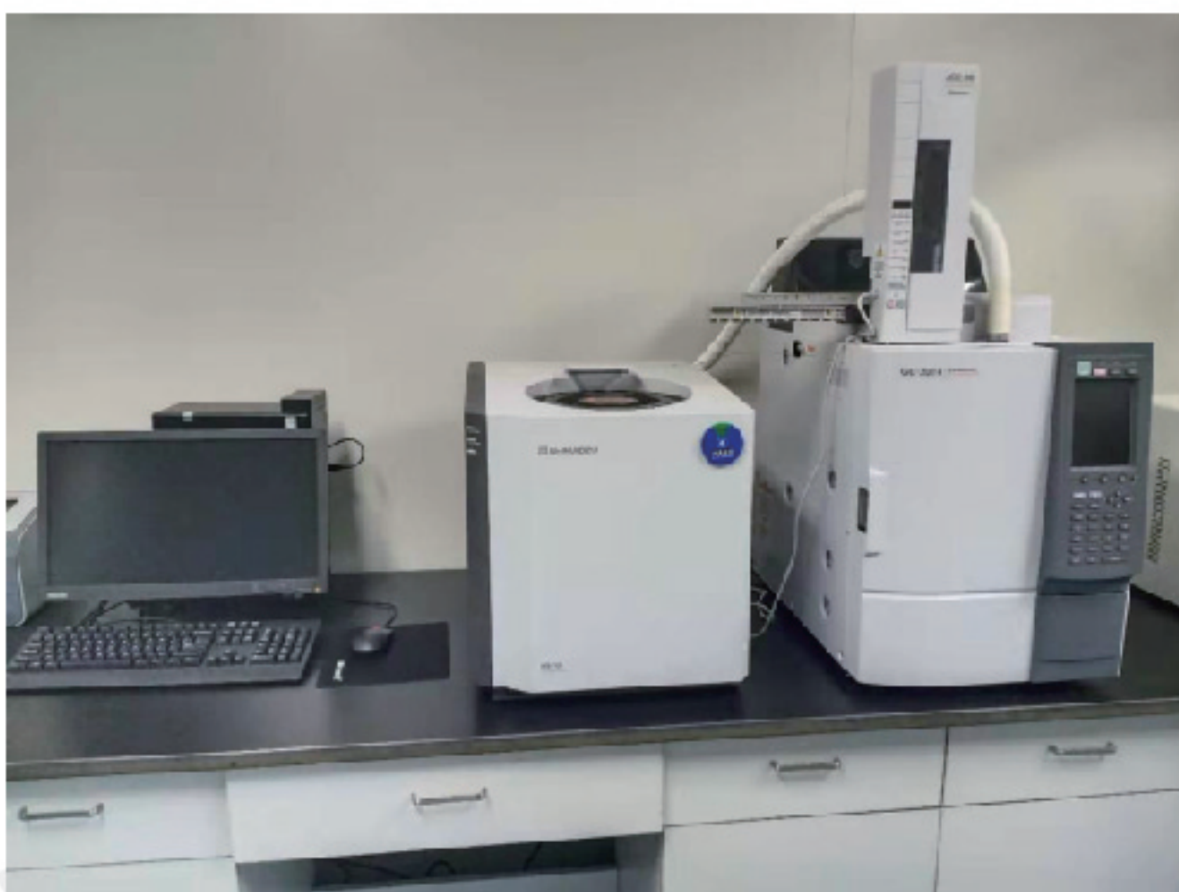
Gas Chromatograph (GC): Applied in flue gas analysis to determine gaseous components.
