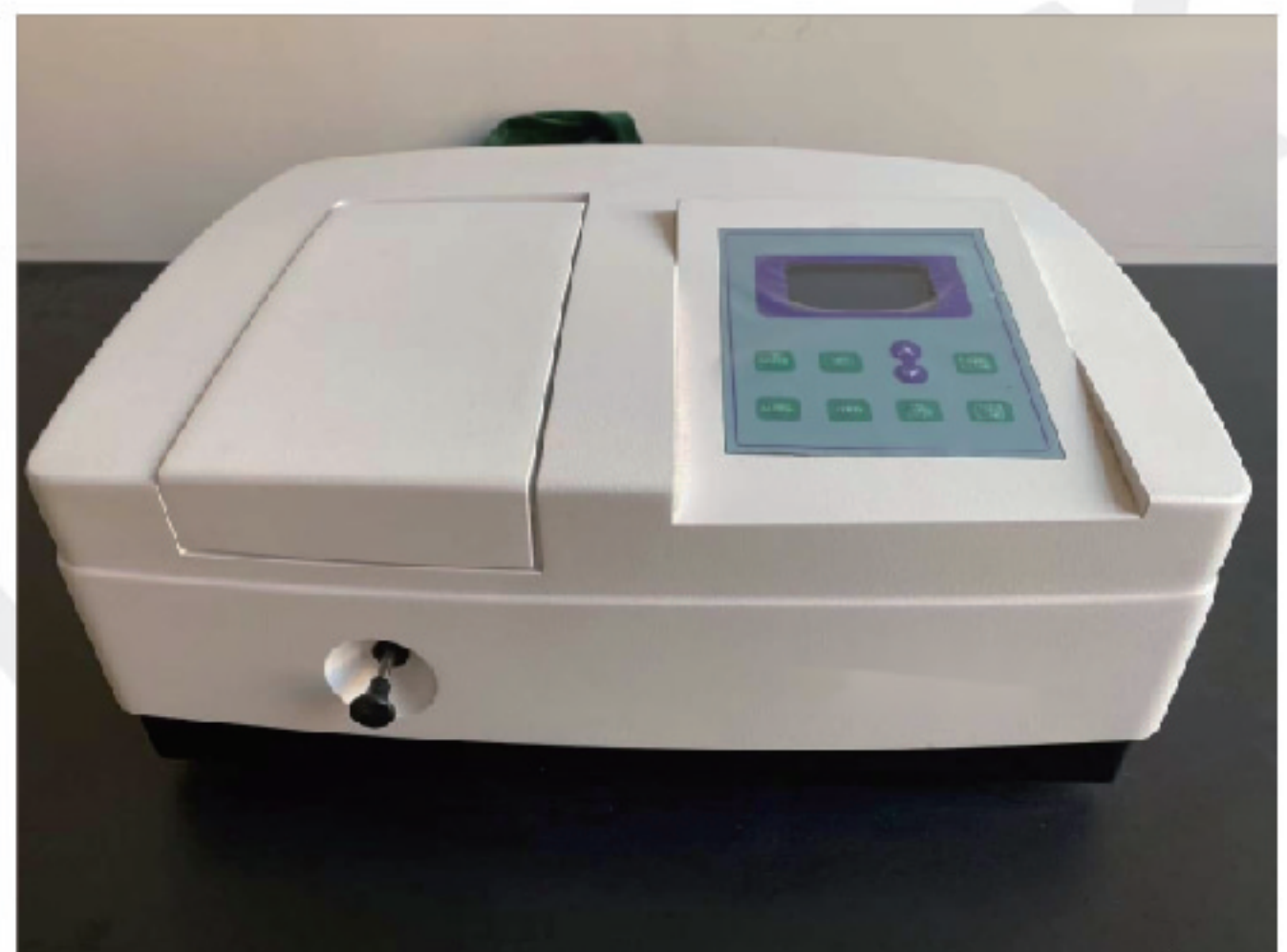
UV-Vis Spectrophotometer: Utilized for liquid analysis, such as quantifying tar or other byproduct compositions.
