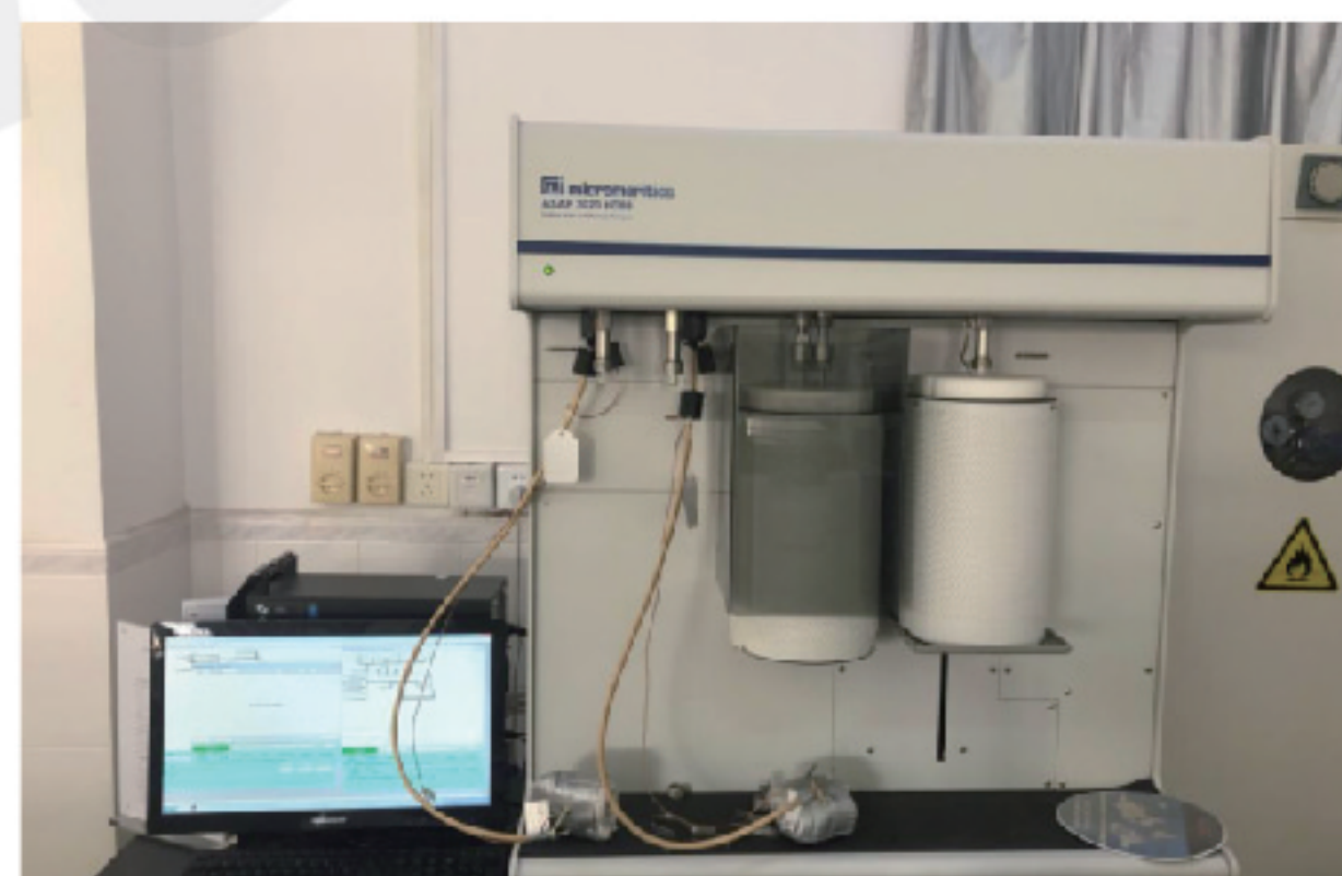
BET Surface Area and Porosity Analyzer: Measures the specific surface area and pore size distribution of biochar, including the proportion of micropores, mesopores, and macropores.
