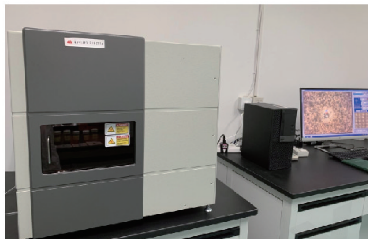
Elemental Analyzer: Used to determine the elemental composition of biochar.
