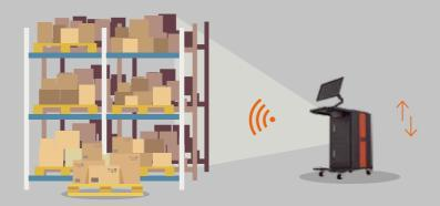
Inventory of cargoes on multilayer shelves is a difficulty of warehousing management. RFID Inventory Trolley is developed by Pinguan to solve such problem. Mainly used in library, archives, small to medium warehouses. It's integrated with a trolley, RFID system and computer system. The RFID antenna can move up and down to identify the cargoes high & low. Compared with barcode scanning, it has the advantages of batch reading, high efficiency, high accuracy based on RFID technology.
