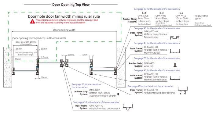
**Application solution**—Hanging sliding Synchronized linkage door
