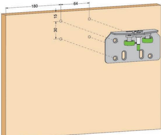
阻尼器安装方向 Damper installation direction
