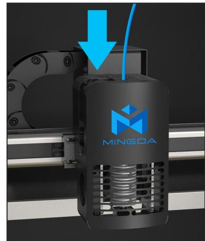
3. Click the heating button
