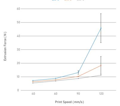
Test parameters: 12mm thick copper heating block, BMG extruder, hardened steel nozzle, nozzle size 0.4mm, layer height 0.2mm.
