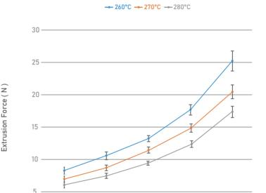
Test parameters: 12mm thick copper heating block, BMG extruder, hardened steel nozzle, nozzle size 0.4mm, layer height 0.2mm.
