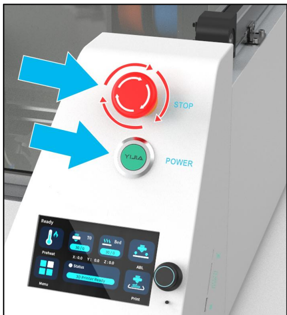
Turn on the emergency stop switch, press the green button to start
