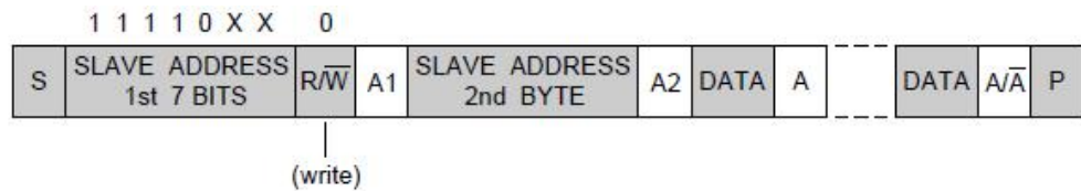
Figure 21- 14 10bit Addressing, Master Writes Data to Slave
