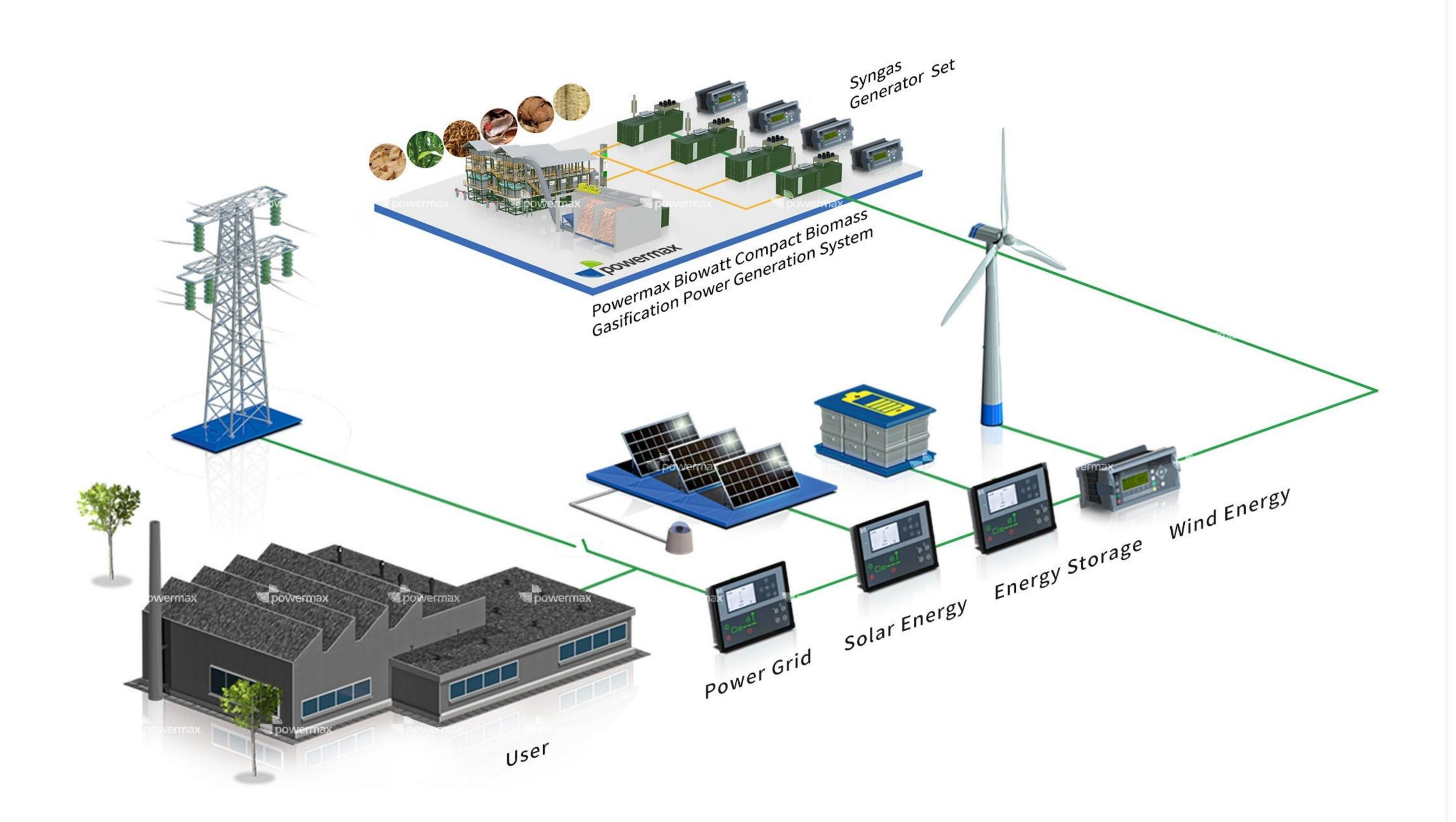
During cloudy days in monsoon season, when solar energy storage plant is forced to idle for lack of sunlight, the biomass power station can continue to generate electricity and feed it into the grid as needed, thereby maximizing the utilization of grid capacity. More importantly, biomass power plants help prevent power bottlenecks and transfer power generation in a timely manner.
