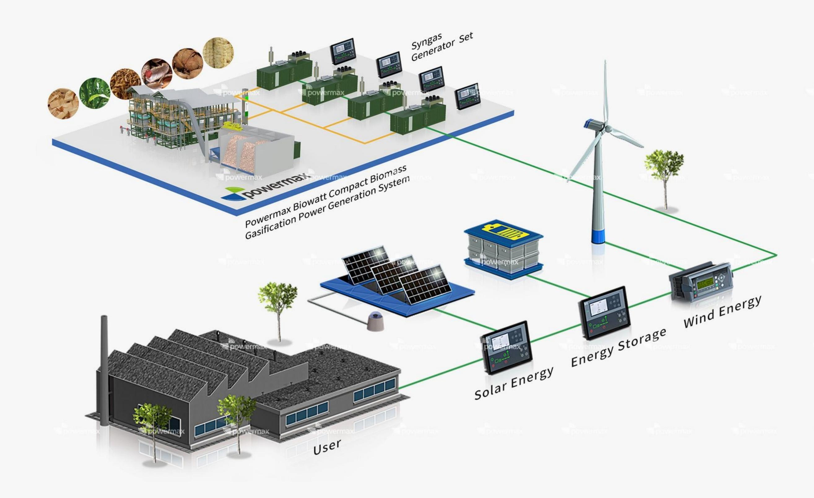
Our hybrid power solutions combine renewable energy sources(such as solar, wind, biomass energy) and energy storage systems together, storing surplus energy and utilizing biomass-powered gasifiers and gas generators to provide instant power replenishment. The hybrid system can make wind and solar power more reliable. Our energy management systems(EMS) can optimize hybrid systems and ensure their reliable operation anytime, anywhere.
