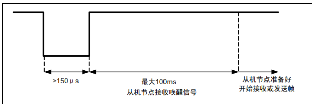
Figure 21-15 LIN bus wake-up signal
