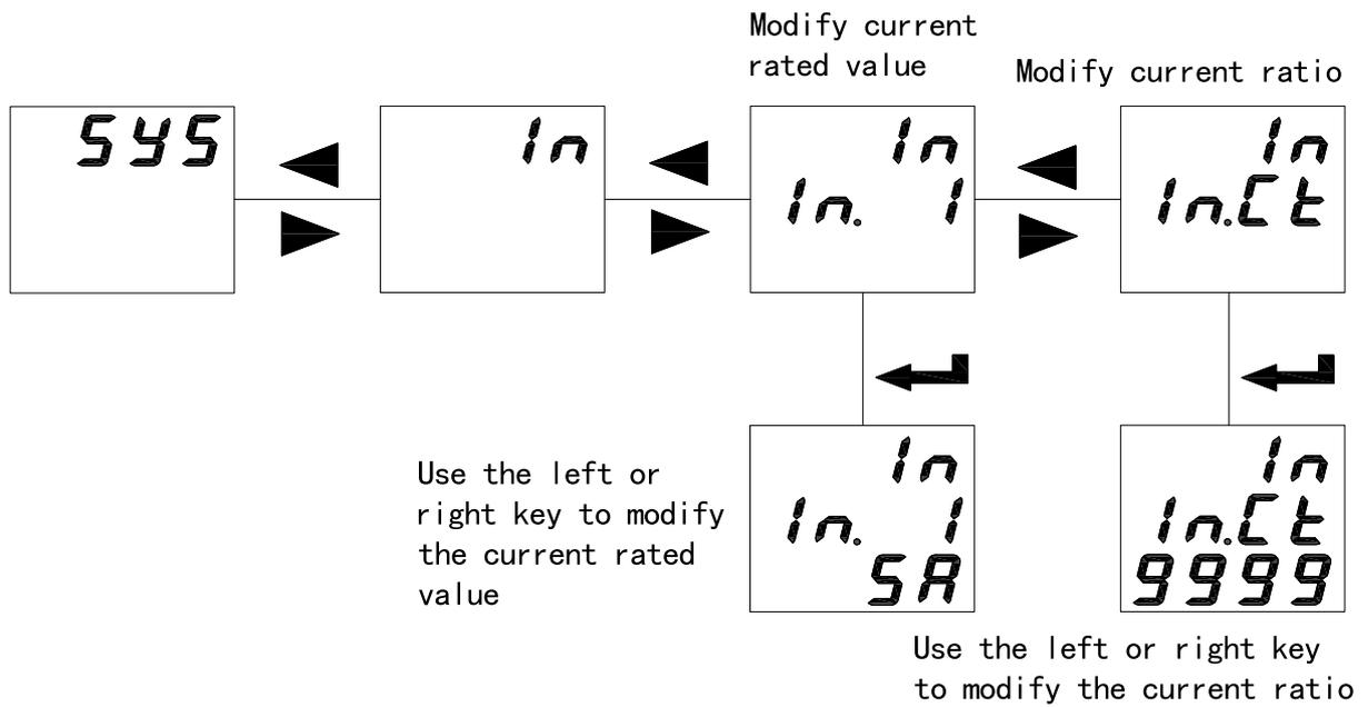
**Note:** IN.I is the current rated value ,IN.U is the input voltage rated value; IN.CT is the current ratio,and IN.PT is the voltage ratio.
