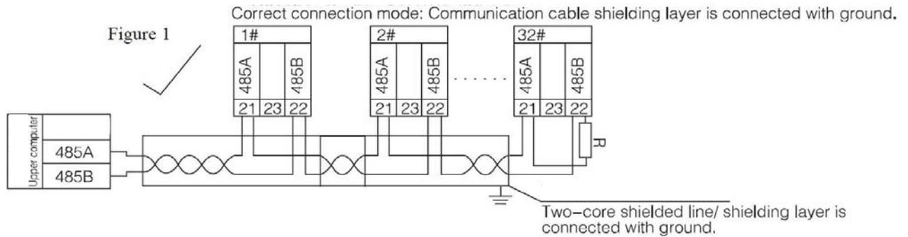
Recommendation of adding matched resistance between A, B of the last meter, the rated resistance range is 120Ω~10kΩ.
