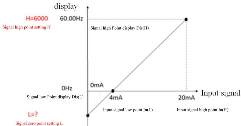
Setting: H: 6000, fi We can get L according to the chart:  $(In(H)-In(L))/In(L) = (Dis(H)-Dis(L))/(Dis(L)-L)$ . So  $L = 0 - (6000-0) \cdot 4 / (20 - 4) = -1500$ .
