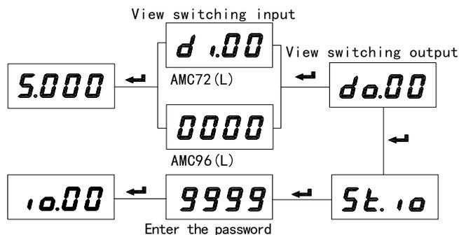
The liquid crystal (LCD) display meter has a switching input/output indication under normal measuring condition,without pressing the shortcut key to look over.
