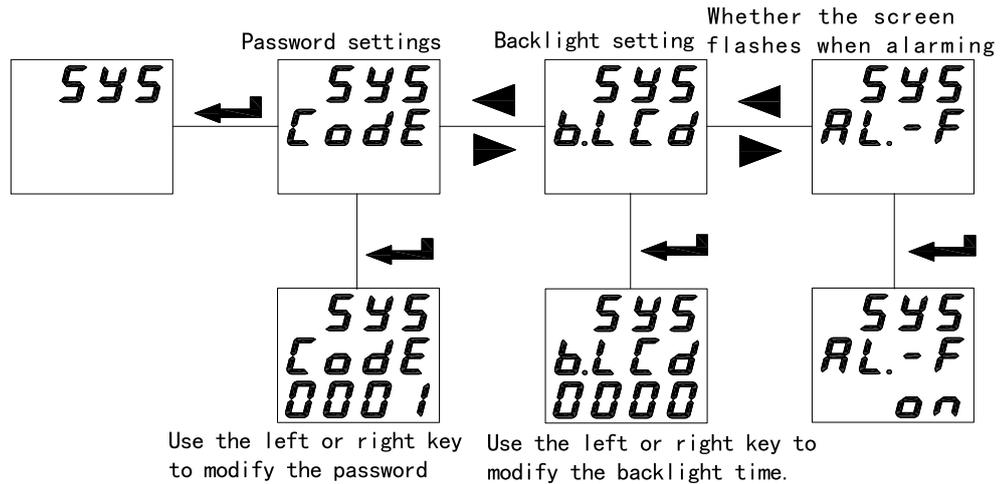
Enter the programming menu, press left or right key to select the LCD page, press Enter key to enter revising condition, left or right key to modify the time to 000 ~ 255s. To LED display meter, this item is invalid.
