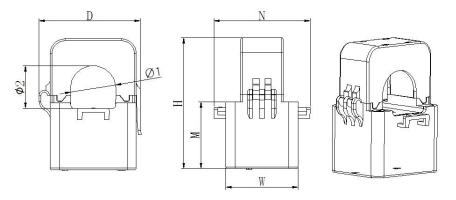
The transformers' secondary outlet wire is single RV lead, whose standard length is  $2m(\pm 10cm error allowed)$ .
