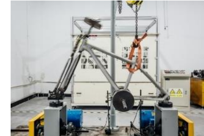
Frame fatigue test
