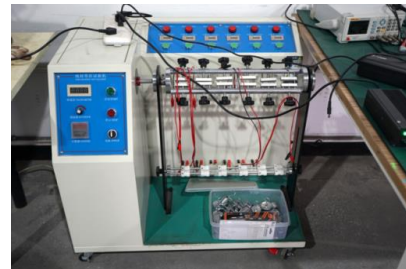
Wire bending test
