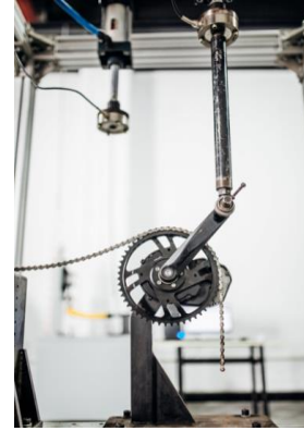
Transmission fatigue test
