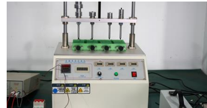
Key lifespan test
