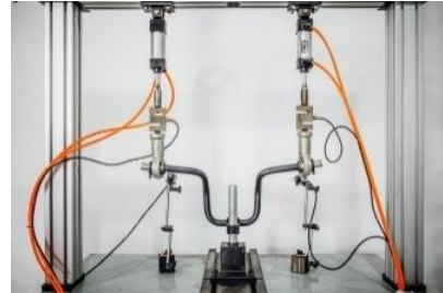
Handlebar fatigue test
