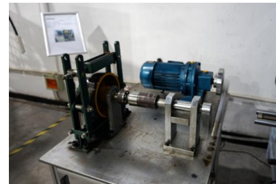
Motor power test
