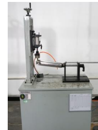
Front fork fatigue test
