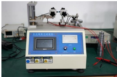
Pulling force test
