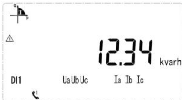
Current forward reactive energy 12.34kWh
