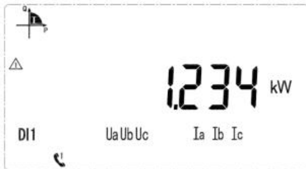
Current total power is 1.234kW
