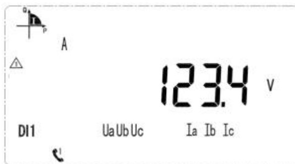
Voltage on A phase is 123.4V
