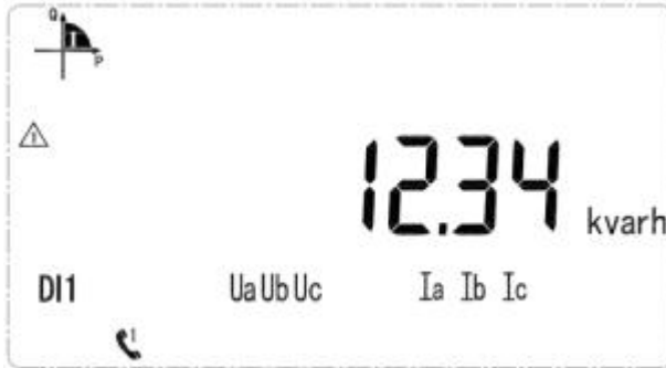
Current forward reactive energy 12.34kWh
