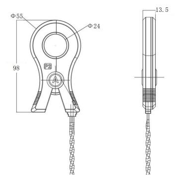
Note: The secondary lead wire of the transformer is a 22AWG dual core wire, with red S1 and black S2.
