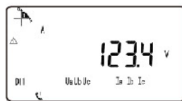
Voltage on A phase
