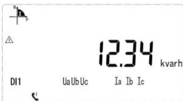
Current forward reactive energy 12.34kWh
