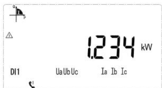
Current total power is 1.234kW
