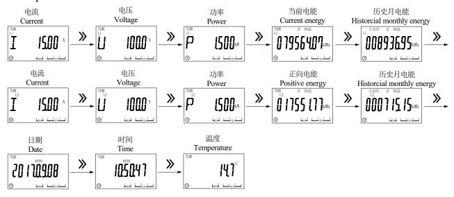
Note: 1. L1 and L2 represent the first and second DC input respectively. When the second DC input is not selected, the L2 parameter interface is not displayed.
