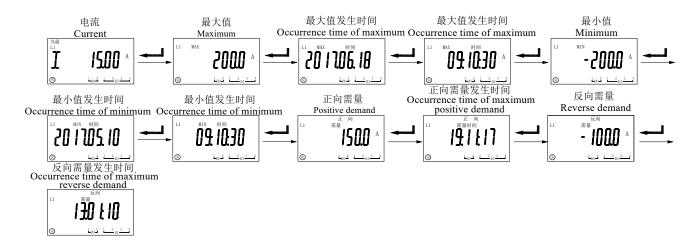
The current display interface is displayed after the meter is powered on, press the right key to switch to the voltage display interface, press the enter key to switch the display: Maximum voltage  $\rightarrow$  Occurrence time of maximum voltage (year, month, day)  $\rightarrow$  Occurrence time of maximum voltage
