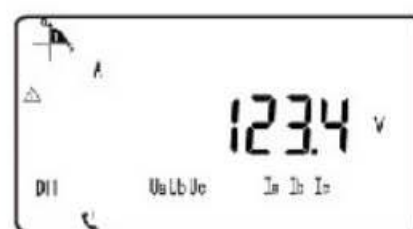
Voltage on A phase
