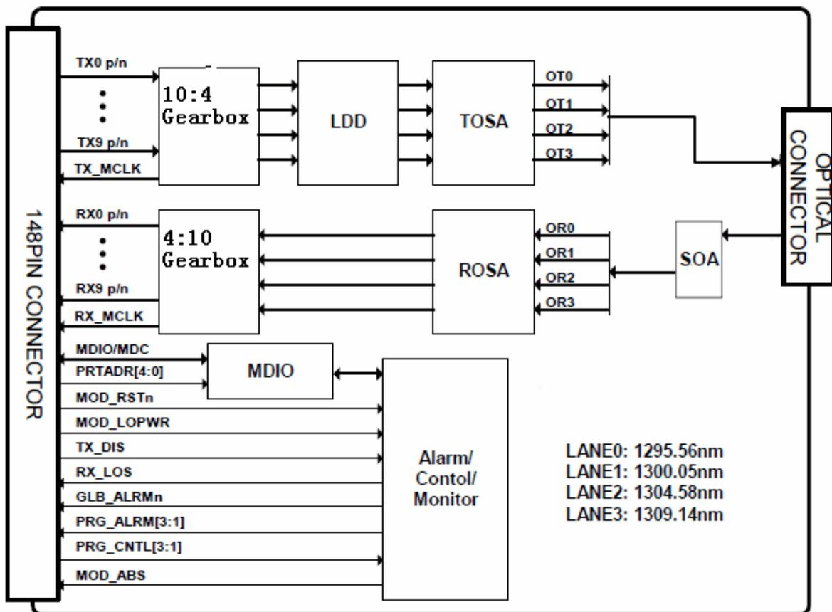
**Figure 1. CFPER4 Optical Transceiver functional block diagram**
